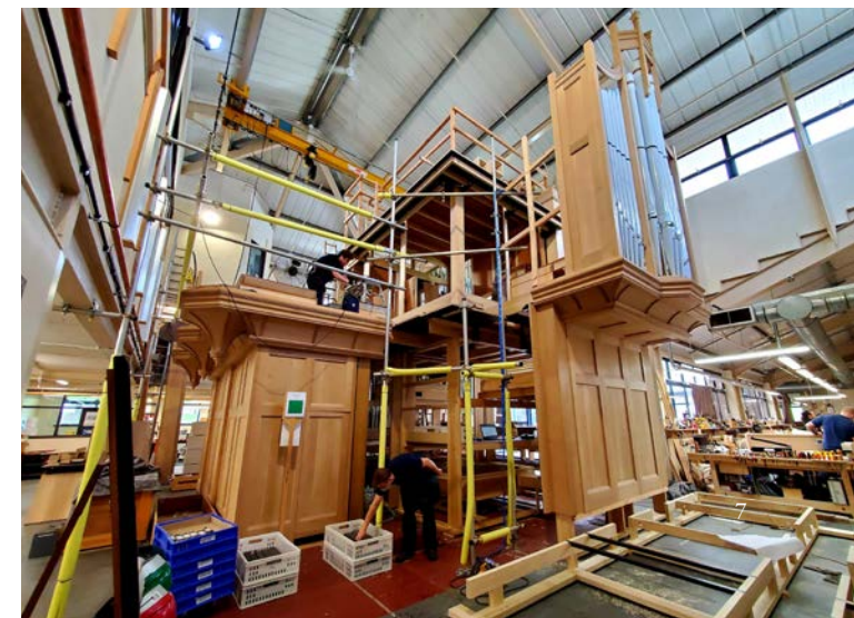
Left: The Great Case frame in place, with some fabric-lined panels installed. Visible at left are the retained 32ft Sub Bourdon pipes, which Harrison & Harrison re-installed several feet higher for improved sound. The Great Case will soon contain pipes of the Great and Pedal Organs, and the Tuba Mirabilis.
